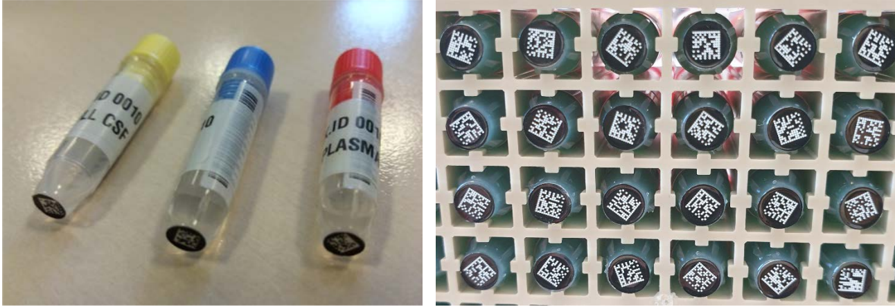
Figure 4. HDClarity biosample vials. 2D barcodes are provided on the vial base (right); Kit IDs are provided on stickers wrapped around the body of the vial (left).
